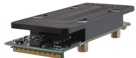
APZU-30x with included heat spreader attached
