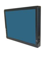
**Argon** offers a versatile 15" rugged display that is particularly suitable for Command & Control applications where space is at a premium such as in combat & tactical vehicles, mobile shelters, and close-in naval spaces. The ARD15's small bezel size, flexible mounting configurations, configurable I/O, and universal AC/DC power supply make it a preferred solution for many mission critical applications.
