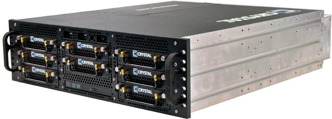
**Field tested, failsafe and long life performance in extreme conditions.** As processing performance continues to improve, Crystal Group is dedicated to minimize the SWaP envelope of the RS378. High-end computing performance in a 3U chassis with a depth of 20" (50.8 cm) fits most any rack space.
