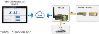
(GUI) are configured with the data acquisition software IPEmotion and automatically transferred to the tablet over WiFi network. The app requires
