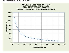
Acumentrics offers user-replaceable, customizable battery packs. With high power density, these are the batteries of choice for many UPS applications. Ideally suited for hot-swap field replacements, these VRLA low maintenance batteries can be mounted in any orientation. They are designed to recharge in an Acumentrics RUPS to 90% in 4 hours, or to 100% in 8 hours.
