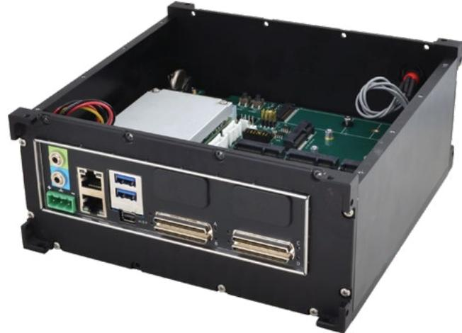
Intel® Atom™ CPU (E3950 Apollo Lake) ♦ Four I/O expansion slots (AcroPack® or mini PCIe)
