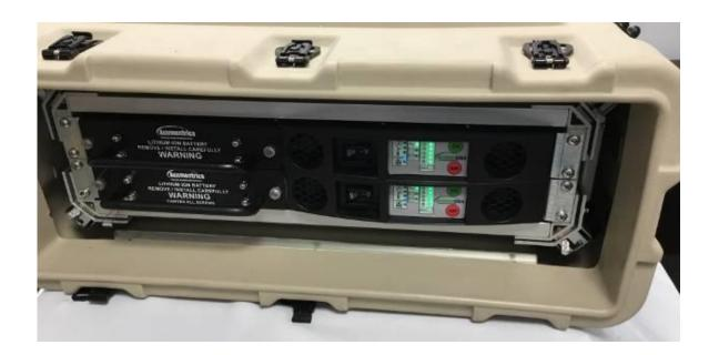
N+1 Fault Tolerant Cable Synchronizes the AC output from both UPS's NO PDU REQUIRED, load shares the AC Output power from both UPS's
