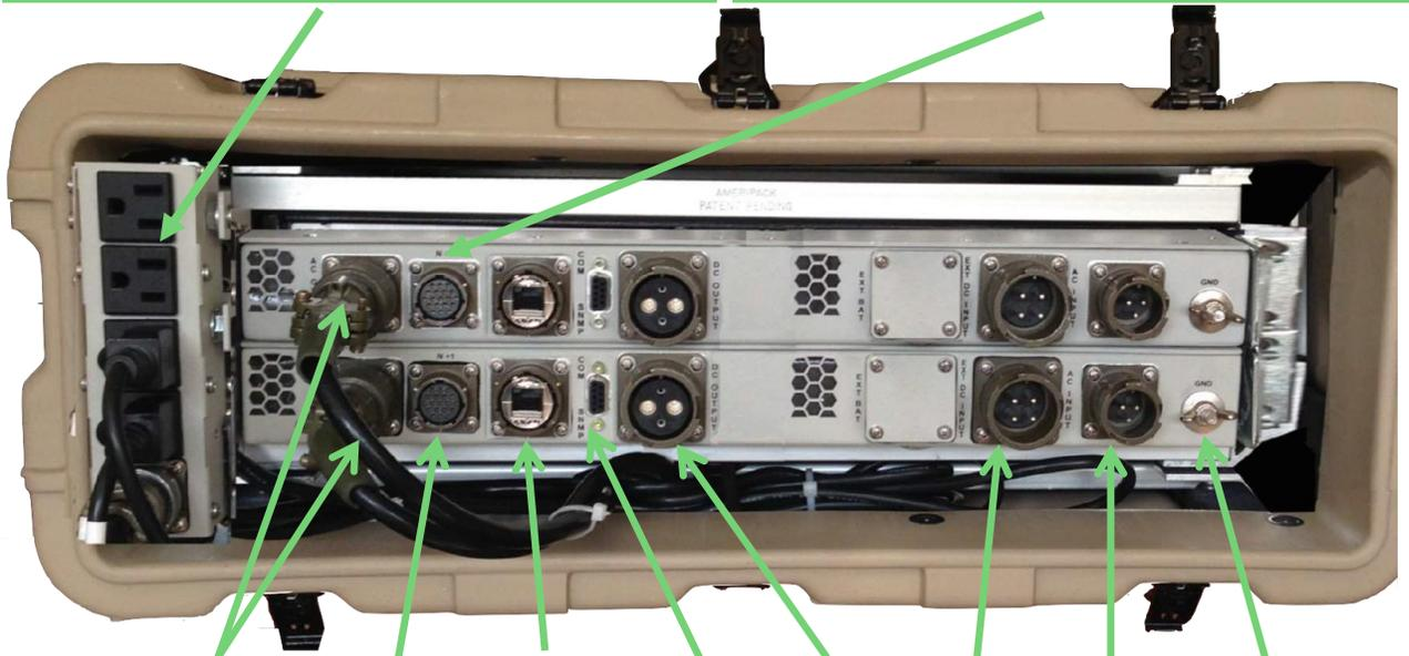
Critical AC Outputs\*\*    N+1 Conn\*\*    SNMP Comm.    RS232 Comm.    DC Output\*\*    DC Input\*\*    AC Input\*\*    Ground Pin
