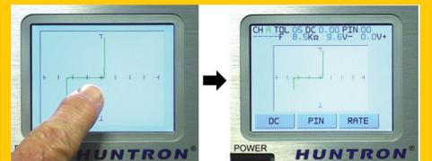
Touching the center of the signature display will toggle the Tracker display between full screen mode and button display mode.
