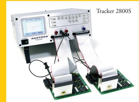
Comparisons between Channel A (green signature) and Channel B (red signature) can take place manually or automatically allowing you to identify signature differences quickly. The Tracker 2800S can save you time when compared to testing with hand probes. You can step through each pin using the touch screen controls, have the Tracker step through the pins at a preset rate or use the optional Huntron Workstation scan and compare for you.
