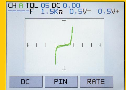
Huntron SigAssist is displayed at the top of the screen and is used to calculate and display numeric values based on the range parameters. The values displayed are resistance (in ohms), capacitance (in farads), power (in watts), and forward and reverse breakdown voltage (in volts).
