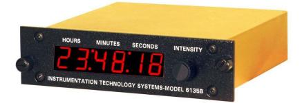
FORM, FIT, FUNCTION REPLACEMENT FOR DISCONTINUED DATUM 9520-647. TESTED & MEETS MIL-E-5400T TESTED & MEETS CE102 PER MIL-STD-461E & RE102 PER MIL-STD-461E POWER, 15-36 VDC 2.0 WATTS. SURVIVES TRANSIENTS PER MIL-STD-704A STANDARD DZUS® RAIL MOUNT PER MS-25212
