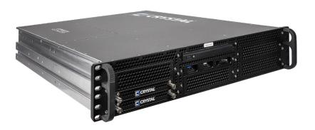
**Field tested, failsafe, and long life performance in extreme conditions.** As processing perfomance continues to improve, Crystal Group is dedicated to minimize the SWaP envelope of the RS255. High-end computing performance in a 2U chassis with a depth of 20" (50.8 cm) fits most any rack space.
