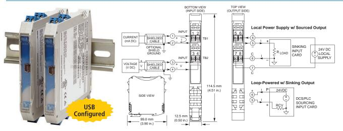
Multi-range ±20mA or ±500mV input ◆ 4-20mA output (sink/source) ◆ 12-32V DC loop/local power
