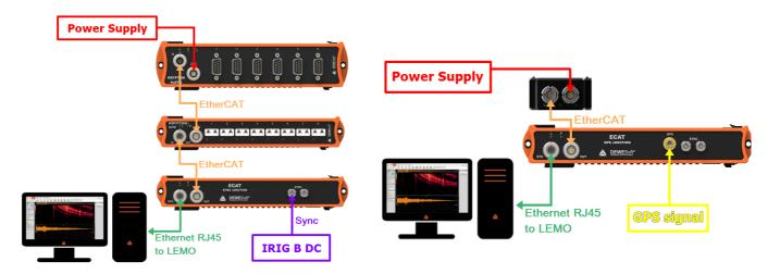
Left system with Sync Junction - Right system with GPS EtherCAT junction
