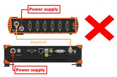
How to **not** connect the PS in ECAT chain
