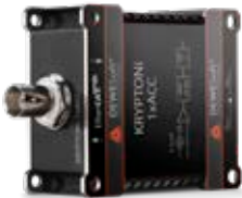
The KRYPTONi-1xACC is a single channel isolated input module that handles virtually any IEPE sensor, providing selectable 4 or 8 mA of constant current sensor supply.
