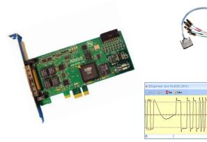
Standard A/D Signal Capture on First Channel
