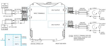
Multi-range ±1V, ±5V, or ±10V input 4-20mA outputs (sink/source) 7-32V DC loop power
