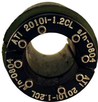
Rotating Fiberglass Collar has embedded Transmitter, Antennas and Inductive Power Circuitry
