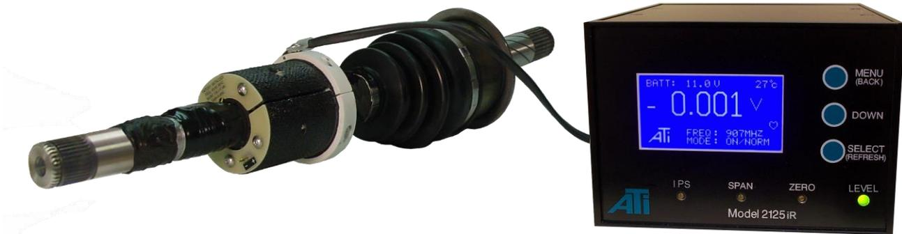
Miniature Digital Half-Shaft Transmitter Collar (attached to half-shaft) shown with 2125iR Digital Receiver
