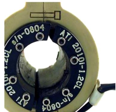
Complete Half-Shaft Collar with 2-Piece Stationary Adapter
