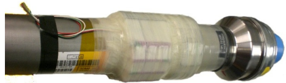
Model 2140LP Transmitter with dual 4-cell AA battery packs shown after final layer of fusion tape has been applied.
