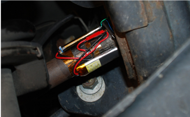
Model 2140LP Transmitter positioned onto shaft
