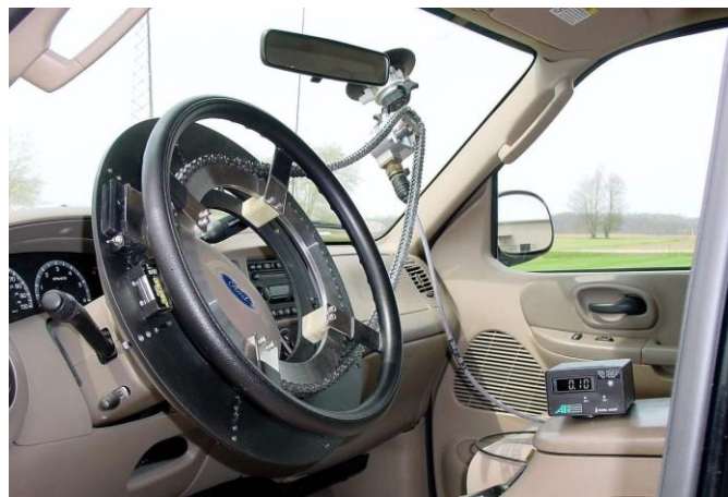
Installed view of Model 2140SE Steering Effort Torque Sensor shown with optional incremental optical encoder.
