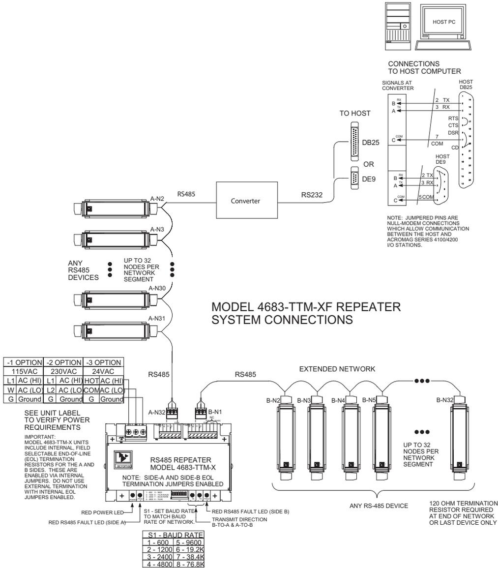
The station configuration drawing is for general illustration purposes only. Johnson Controls system customers should instead refer to the Metasys® Network Technical Manual for N2 Bus Communication, or the MS/TP Communication Bus Technical Bulletin for wiring connections using the 4683-TTM-xF repeater.
