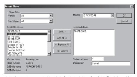
Step 2: The network management software (SyCon from Lantronix shown above) lists Profibus devices available for configuration after their GSD files are copied to the software's directory using Windows Explorer.
