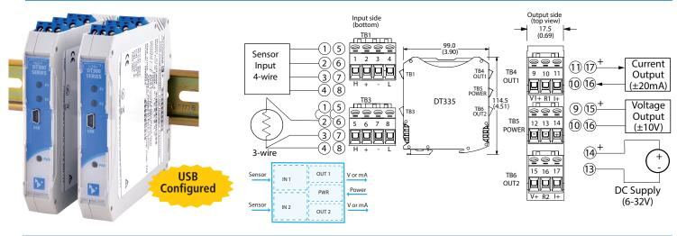
Dual channels ◆ RTD (Pt, Ni, Cu) or 0-4500 ohm input ◆ 0-20mA, ±10V outputs ◆ 6-32V DC local/bus power
