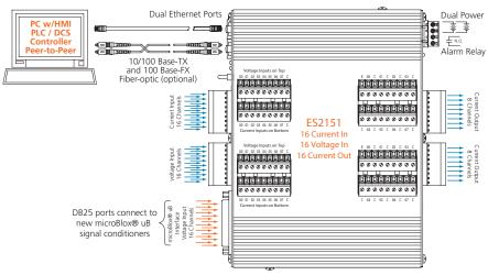
32 analog current/voltage inputs ◆ 16 analog current outputs ◆ Modbus TCP/UDP, i2o communication
