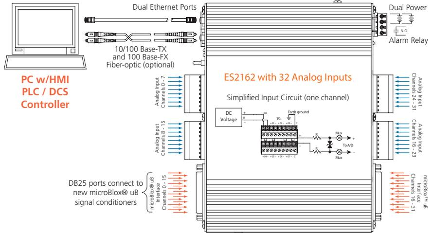
32-channel differential analog voltage input with uB interface ♦ Modbus TCP/IP or UDP/IP communication
