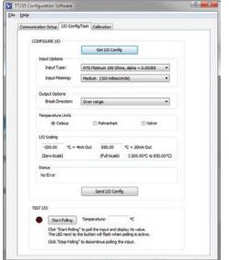
TT235 Model software allows you to configure transmitters offline. save the file, and download into units later, at your convenience.
