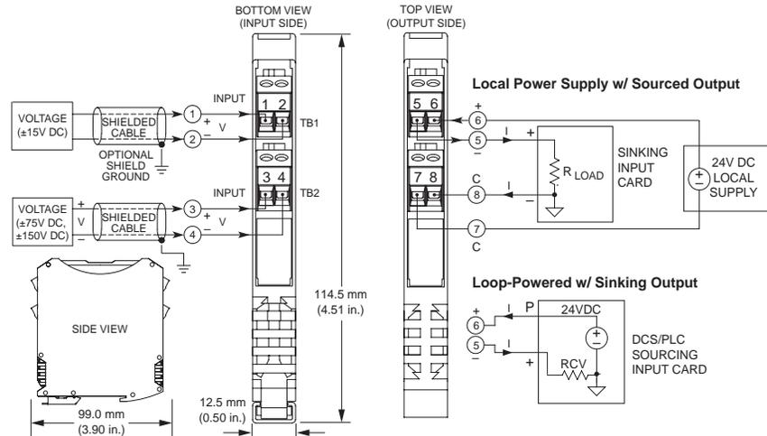
Multi-range  $\pm 15V$ ,  $\pm 75V$ , or  $\pm 150V$  input ◆ 4-20mA output (sink/source) ◆ 12-32V DC loop/local power
