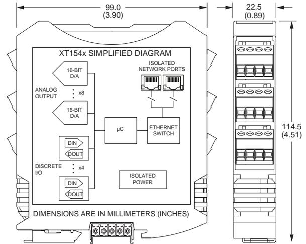
8 analog voltage outputs, 4 discrete I/O channels ♦ Modbus TCP/IP, Ethernet/IP, Profinet, or i2o communication
