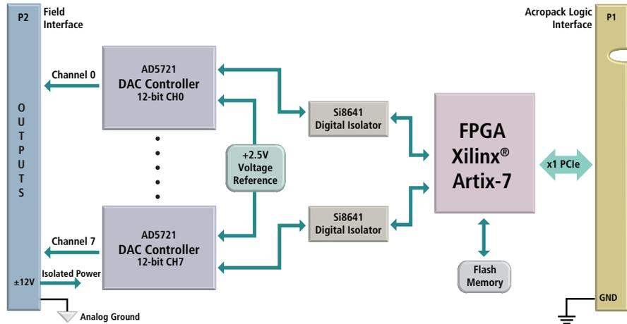
12-bit DAC ◆ 8 Channels Voltage Output ◆ Wide Temperature Range ◆ PCIe Bus Interface
