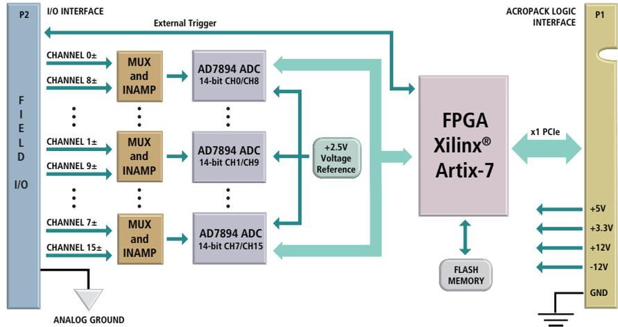
14-bit ADC with Simultaneous Multi-channel Conversion ♦ Wide Temp. Range ♦ PCIe Bus Interface
