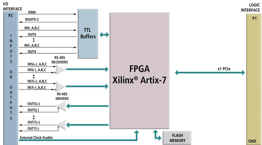
Eight 32-bit Counters ♦ TTL and RS422/RS485 I/O ♦ Wide Temperature Range ♦ PCIe Bus Interface
