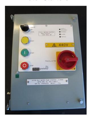
The Gresham Range of Motor Starters are 440V I/P and O/P with under-voltage and phase rotation protection. They also incorporate trip functions derived from the motor.
