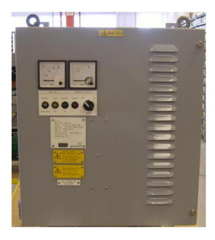
The Transformer Rectifier Unit type 3RC1KB provides a high quality output of 27.4 volts dc when used for float charging valve regulated lead acid batteries or can be set for 24V for ships 24V systems.
