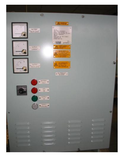
The 1D1000B30C Uninterruptible Power Supply (UPS) provides a high quality output of 115v 60hz  $1\phi$ @ 1000VA from an input of 115v 50/60hz. The integral valve regulated lead acid battery will support the output for 30 minutes in the event of an input supply failure.
