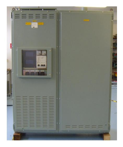
The 1RPQ10KB30A Uninterruptible Power Supply (UPS) supplies a battery supported ,115V, 60Hz single phase output to ships loads. The UPS consists of a transformer isolated rectifier, battery and an inverter.
