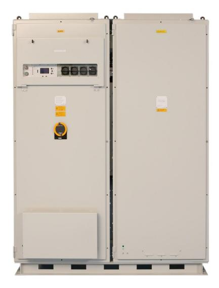
The 3RPQ15KB30B Uninterruptible Power Supply (UPS) supplies a battery supported ,230V, 60Hz three phase output to ships loads. The UPS consists of a transformer isolated rectifier, battery and an inverter.
