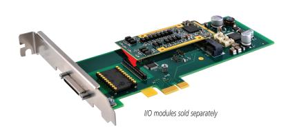
One AcroPack or mini-PCIe mezzanine module slot
