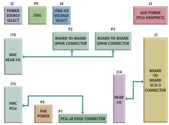
One XMC mezzanine module slot ◆ Non-Intelligent carrier card ◆ PCIe x8 interface
