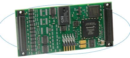
These modules support adaptive computing applications with an FPGA running custom programs to control system communication.
