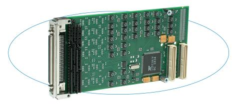
With eight serial ports per module, the PMC521 provides a high-density solution to reduce costs and use fewer card slots.
