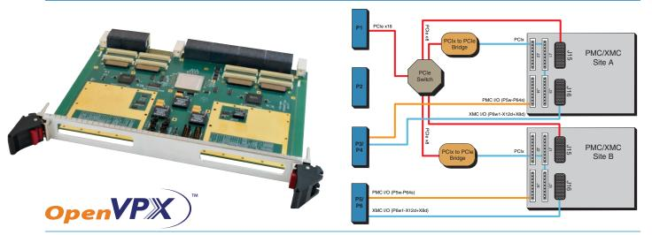
PCIe x8 Gen 2 interface via Data plane ◆ Two PMC/XMC slots ◆ 6U form factor
