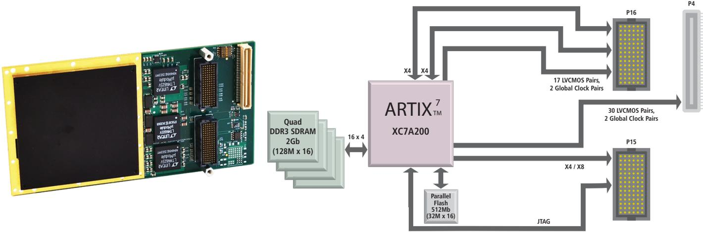
XMC module with PCIe interface ◆ Logic-optimized Artix-7 FPGA ◆ Conduction-Cooled
