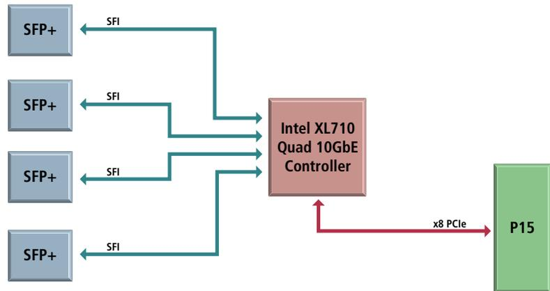
Quad SFP+ ports ♦ Intel® XL710 Controller ♦ PCIe Gen 3 x8 interface ♦ Extended temperature operation
