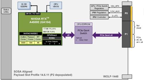
SOSA aligned model with support for Payload Slot Profile 14.6.11-0. The P2 connector is depopulated for this model.
