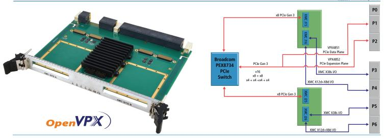
Two XMC slots ◆ PCIe x16 Gen 3 interface via Expansion or Data plane ◆ Air or Conduction-cooled
