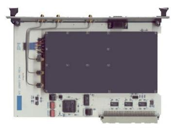
The Lumistar LS-25-V Receiver is a single-band, single-slot VME FM Receiver. Versions are available for P-Band, Lower L-Band, Upper L-Band, S-Band, and NATO E-Band depending on the model chosen. These wideband designs support PCM data rates up to 20 Mbps and include both an FM demodulated output for PCM data, and AM and AGC/RSSI outputs. DC coupling is employed to ensure a high quality data link with long strings of NRZ-L ones or zeroes.
