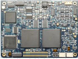
pseudo-random patterns and calculate internal bit error rates with or without the injection of forced errors. Various status indicators are also available through the software. The Bit Synchronizer also contains a BER reader as well as frame sync pattern indicator.
