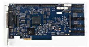
The IRIG Time Code Reader and Generator operate with IRIG A, B, or G time codes. The Time Code Reader is typically used to insert time information into the PCM minor frame block of data. The Time Code Generator creates and outputs time information in accordance with the IRIG Time Code Standards. Both reader and generator are capable of operating at  $\frac{1}{2}$ , 1, and 2 times the normal rate.
