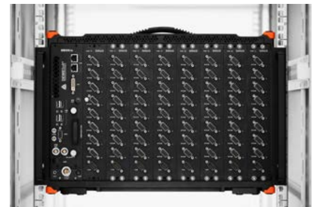
Figure 5. R8rt is a high-channel-count DAQ system with high-end signal conditioning, powerful computer, SSD data logger, and low latency data output capability to 3rd party EtherCAT real-time controllers.
