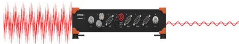
Figure 8. SIRIUS as a standalone signal conditioner.
