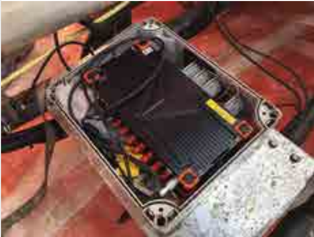
Figure 6. Test of housing using SIRIUSi slice under the driveshaft.
