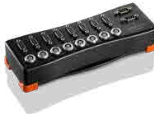
Figure 2. DEWE-43 data acquisition system.
