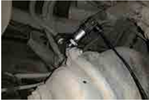
Figure 5. Pressure sensor installed in the brake chamber with tee coupling.
