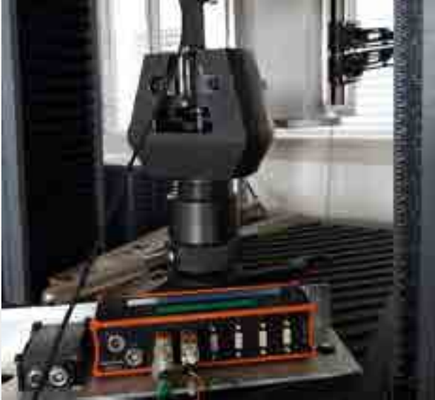
Fig. 14. Krypton modules are used to calibrate dummies and sensors.
