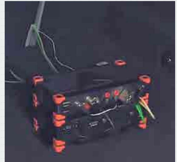
Figure 2. The high-speed DAQ SIRIUS reliably performed excellent services in the trunk of the M5, while robust Krypton modules digitized the engine's sensor signals.
