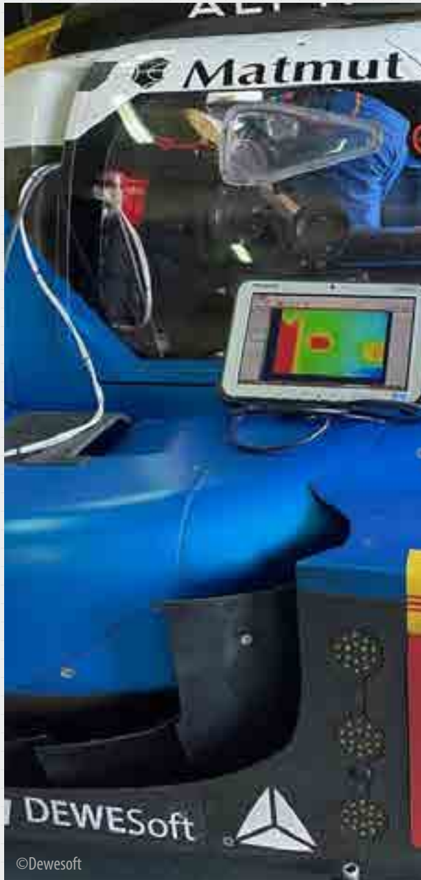
Figure 3. Using Dewesoft and an Optris infrared camera to measure temperatures inside the cockpit.
