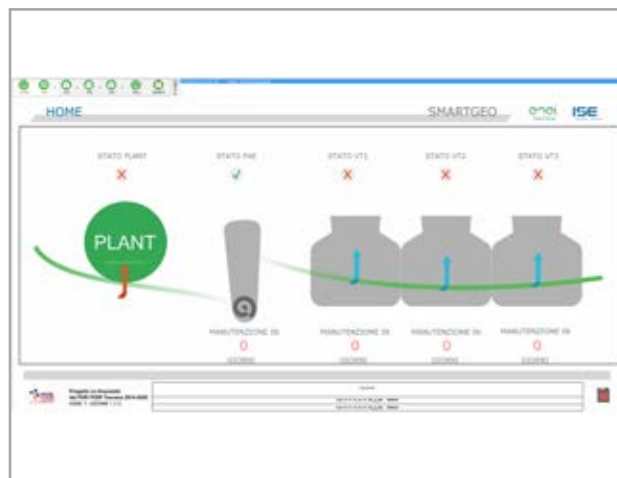
Figure 6. PAE pump monitoring screen
