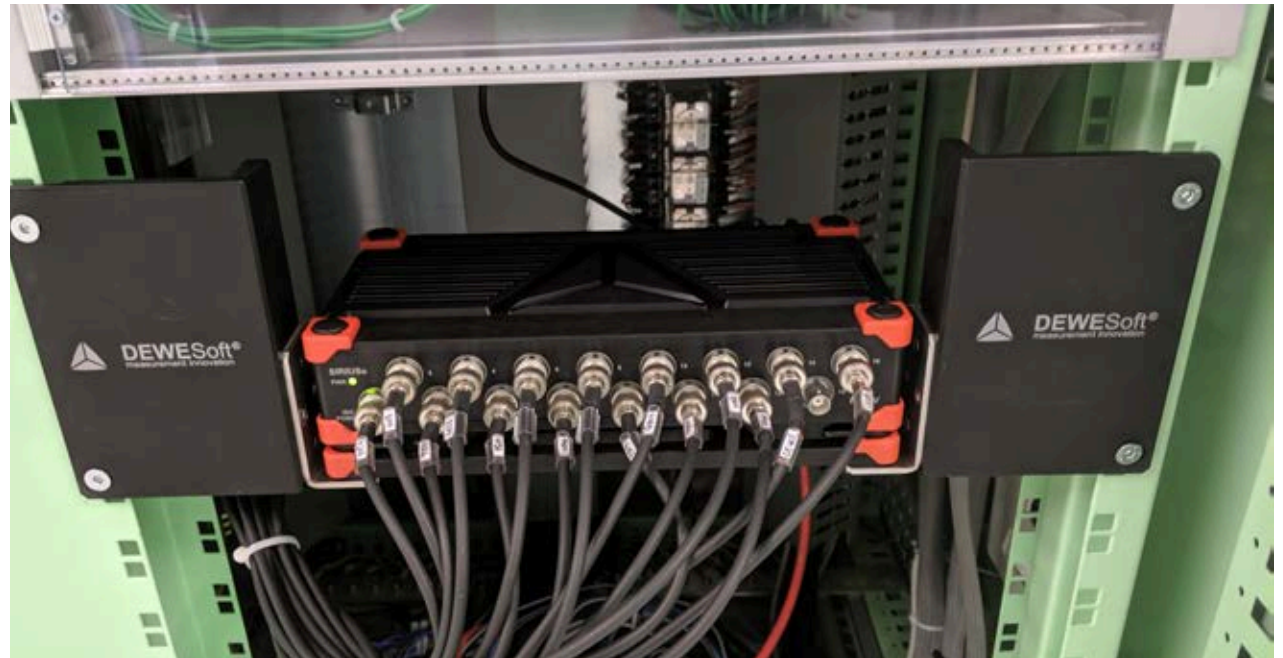
Figure 4. The Sirius data acquisition system acquires a signal from the main turbine (picture above) and the generator.
