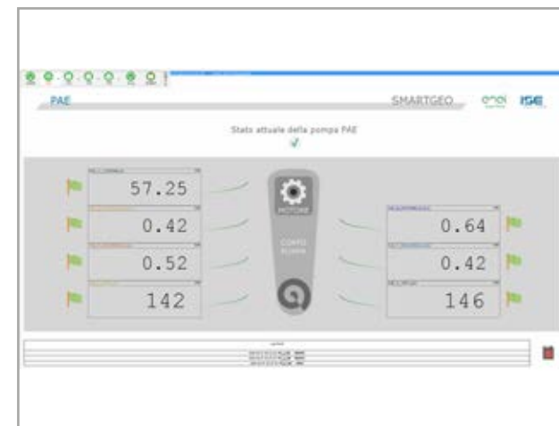
Figure 7. PAE Pump bearings analysis (using envelope detection algorithm).
